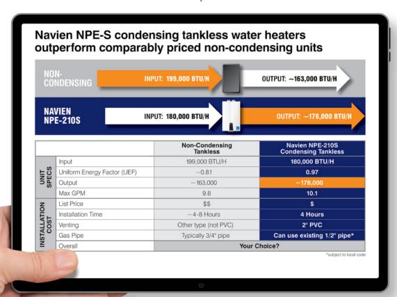
The NPE-S condensing tankless water heaters are so efficient that they outperform much larger capacity non-condensing competitors. More output for the money, lower installation costs and lower operating costs for customers makes it a smart choice.
